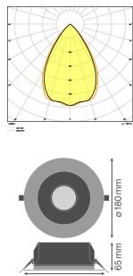
**Scheda tecnica Ledvance Downlight LED Performance DN155 14W 1500lm 65D - 830 Luce Calda | 180mm - IP54**
