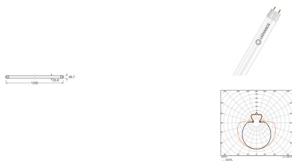
**Scheda tecnica Ledvance Tubo LED T8 EM Value Conventional (EM), Mains (AC) Standard Output 15W 1800lm - 840 Bianco Freddo | 120cm - Sostitutiva 36W**
